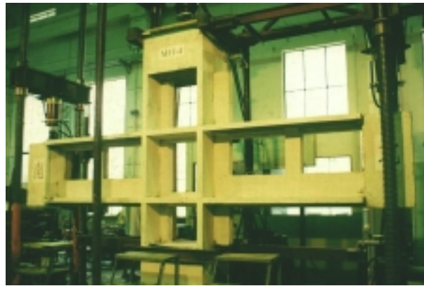
Fig. 3. Joint Specimen and Test Setup
